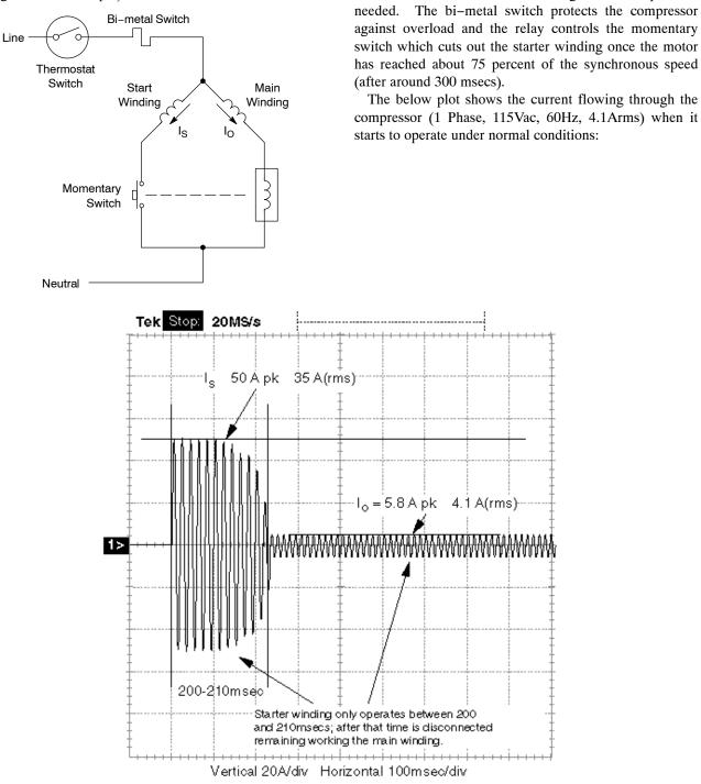
This plot shows the total current flowing through the compressor when it starts to operate and the time in which the current reaches the maximum value (Is) due to the start of the motor. After this time (210 msecs) the start winding
