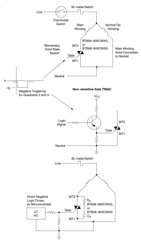
In the first diagram, the triac BTA08–600CW3G or BTB08–600CW3G is making the function of the conventional relay's momentary switch, and it can be triggered by using a transistor as shown in the above schematic or through the signals of a microcontroller. Since this triac BTA08–600CW3G or BTB08–600CW3G is a snubber–less device, it does not need a snubber network for protecting itself against dV/dt phenomena.
