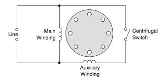
When the line voltage is applied, the current flows through both windings and the result is a rotating stator field which causes the motor to start. At about 75 percent of synchronous speed, the auxiliary winding is cut out by a centrifugal switch. The following figure shows a conventional schematic diagram using a relay for controlling a split–phase fractional horsepower motor (the compressor of a refrigerator for example):
